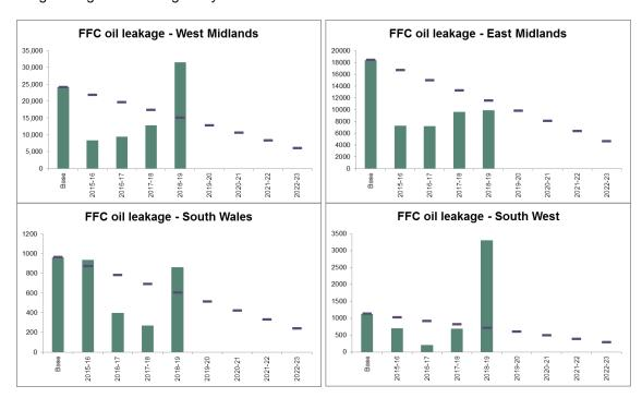
**5.156**In the West Midlands two circuits contributed to 67% of leakage. Perfluorocarbon tracer (PFT) was used to enable leak location and these cables have now been fully repaired.
